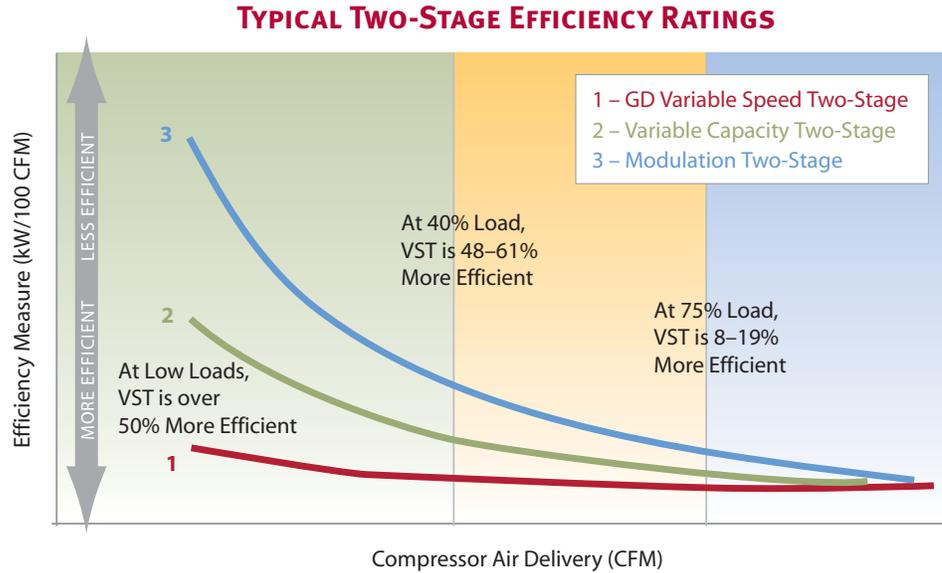
compared to the other compressor types. The VST compressor offers up to 61% better energy efficiency than other compressor manufacturers, and the advantage increases as flow demand decreases.
